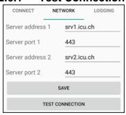
After entering the connection type and the network properties, the connection can be checked by clicking on the button "TEST CONNECTION".
